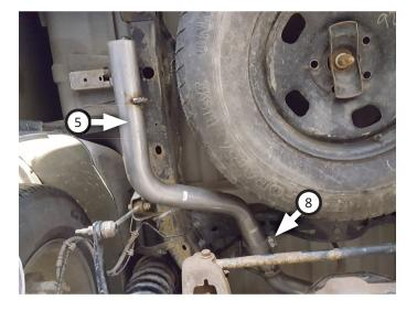
12. Place clamps (x2) (8) onto rear exit pipes (6) then connect them to tailpipes. Tighten clamps enough to allow for adjustment.
