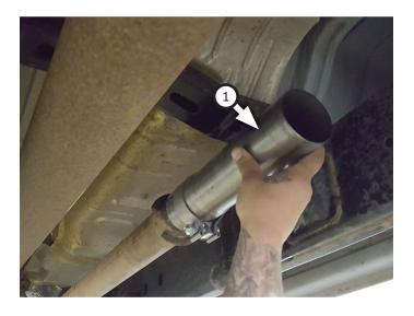
Place clamp (9) onto AMT muffler (2) then connect it to adapter pipe. Tighten clamp enough to allow for adjustment then place clamps (x2) (8) onto muffler outlets.
