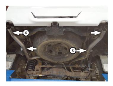
13. Place **stainless tips (7)** onto both exit pipes and adjust to desired position. Tighten pinch clamps enough to hold in place.
