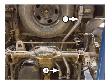
11. Place **clamp (8)** onto **left rear tailpipe (5)** and connect it to left front tailpipe. Set wire hanger at rear of tailpipe into isolator as shown, then tighten clamp just enough to allow for adjustment.
