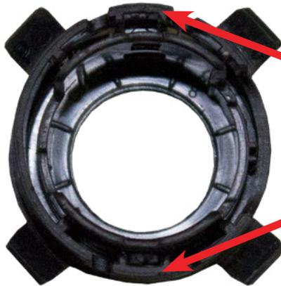
Spread these tabs and release the outer mounting ring from the rear
