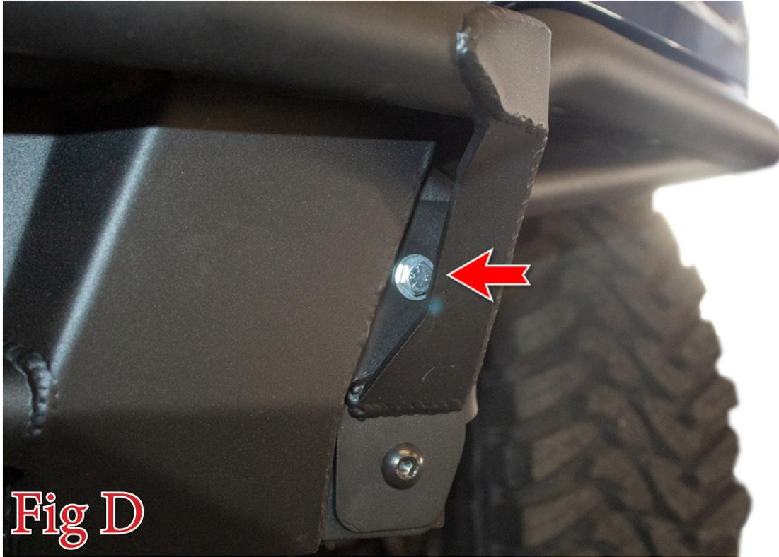
5. Torque the 3/8" Mounting bolts to 30 foot pounds, and the 1/2" Mounting bolts to 70 foot pounds.
