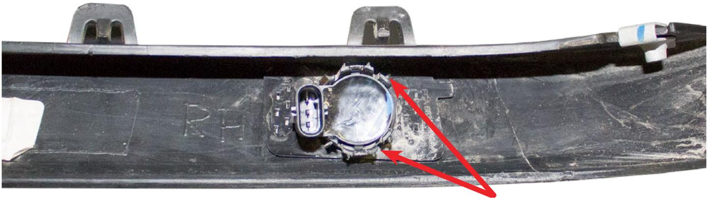
**Release the parking sensor by spreading these two tabs**
