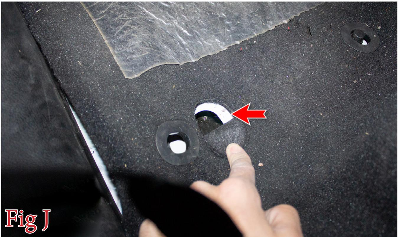
14. One person will need to send the harness up through the hole in the bottom of the body (shown in Fig K) as someone else grabs the harness from the top (through the hole you just removed the rubber plug out of). **Keep the wiring away from the exhaust.**
