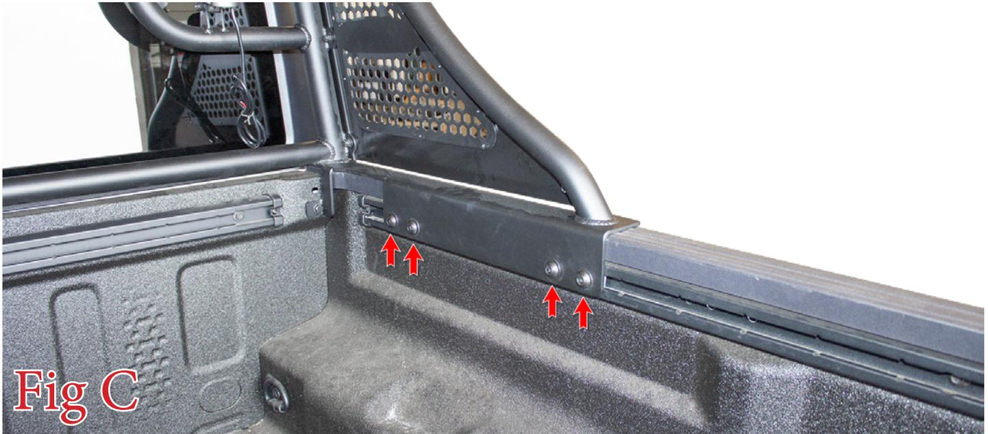
5. If your vehicle does not have the factory bed rail option and you have the additional mounting kit, follow this step. With the chase rack sitting in place on the vehicle, put the Mount Kit Plate in place so that your bed rail gets sandwiched between the Chase Rack and the Mount Kit Plate. Use the supplied 1/2" Bolts and Washers (4 per side) that come with the chase rack along with the 1/2" Washers and Nuts (4 per side) that come with the Mount Kit to secure it. (Fig D)
