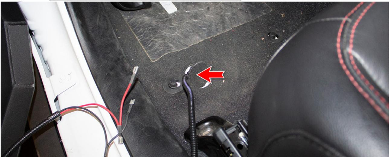
15. Cut a slit in the rubber plug you removed in Step 13. Then, pass the harness through that slit and reinstall the rubber plug in its original location. (Fig L)
