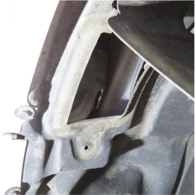
5. Remove the 10mm Bolt that sits inside the access panel you just opened. Do this on both sides of the vehicle.
