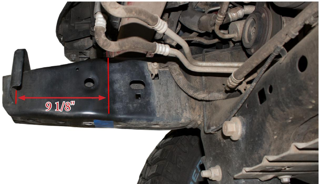
9. Make sure the two tabs on the bumper mounting brackets can sit flush against the truck's body mount. If they do not sit flush against that mount, you will need to grind more metal off the frame. Once your cuts are final, make sure to paint over any exposed metal. (Fig I)
